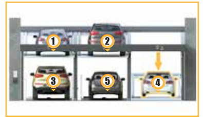
Then platform #4 is lowered to the entrance level.
